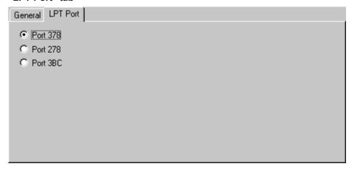
There are three port address options. These echo the standard PC interfaces LPT1, LPT2 and LPT3. Your PC manual will tell you which LPT port on your computer corresponds to which port address. Alternatively check the current BIOS setting.
