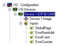
The CIF-30 automatically provides four input bytes which describe the status of the card and the CAN bus:
