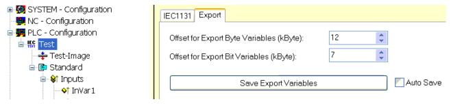
In fig. 3 the start address for PLC variables created in this manner is changeable, calculated with binary prefixes. In fig. 3 the start address is at 7 KB =  $7186_{dec}$  bytes =  $E000_{hex}$  bytes.
