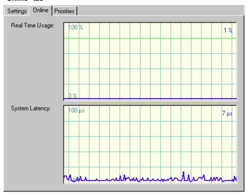
The online display gives information about the current CPU load. This is the amount of time required by the real time task. The bright green line indicates the pre-set *CPU Limit* value.
