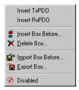
The menu alongside is obtained by right clicking on the general CANopen node. Here you can insert further Tx PDOs and/or Rx PDOs.
